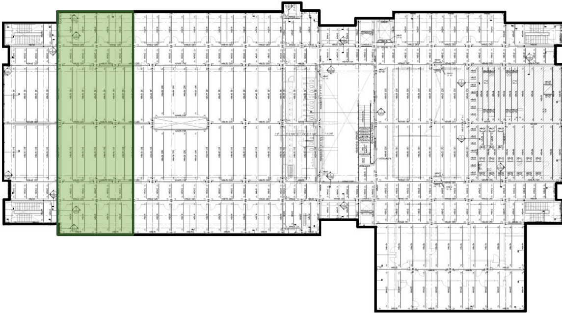
Figure 1: Typical Bay Chosen for Structural System Estimate
